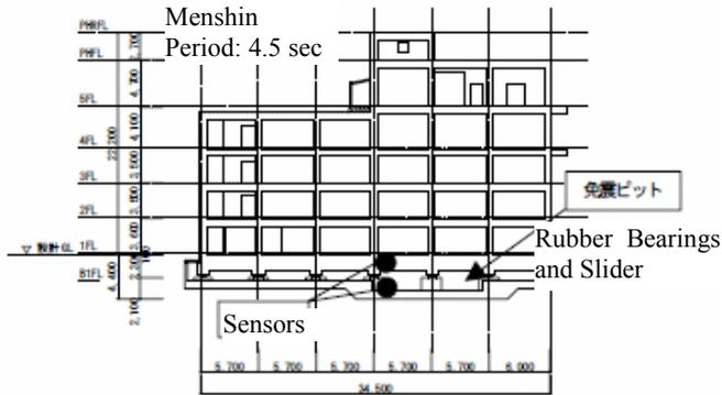
Fig.6.2(a) Elevation of the structure
