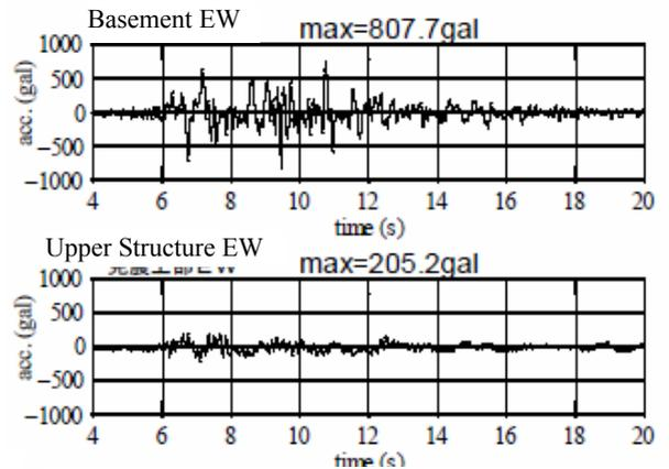
Fig.6.2(b) Observed Accelerations(EW Direction)
