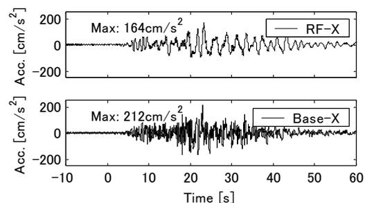
Fig.6.1(b) Observed Accelerations(X Direction)
