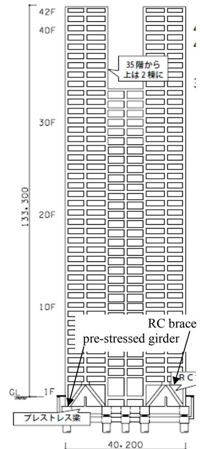
Fig.4.1 (b) Elevation of frame
