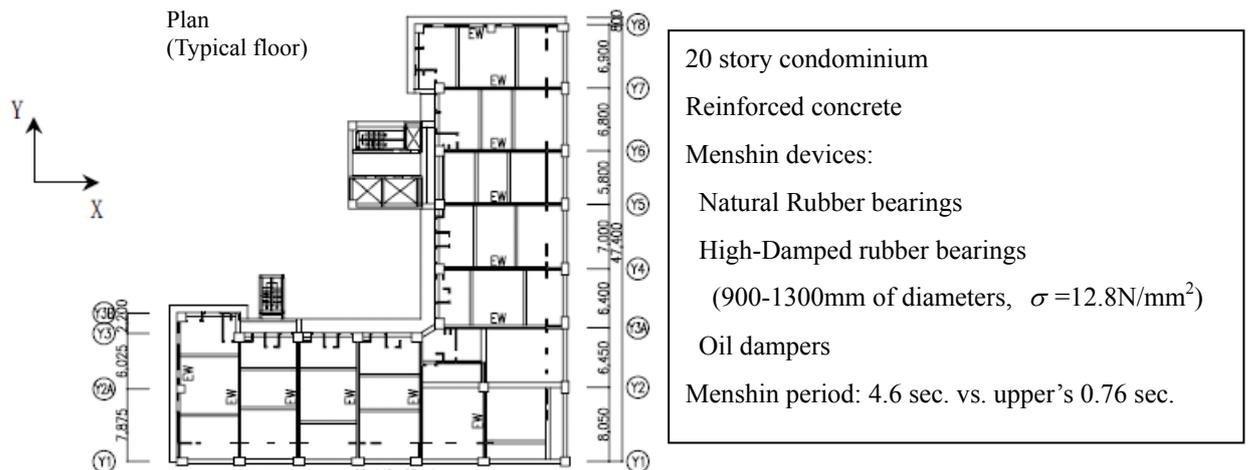
Fig.4.3 L-shaped plan with intermingled moment resistant frames and shear walls
